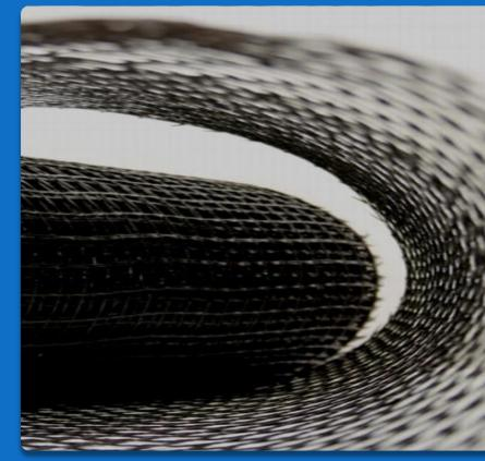
Reinforcement of plaster layers inside and outside the building helps form the internal frame layers and provides excellent retention and protection of the plaster layer.
